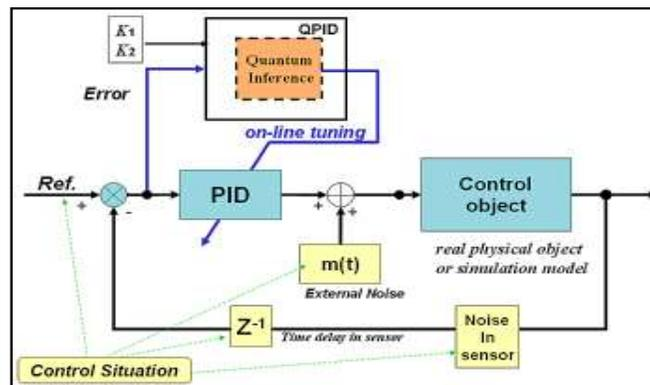
Figure 1. General structure of QPID based on two K-gains of classical PID and quantum inference
