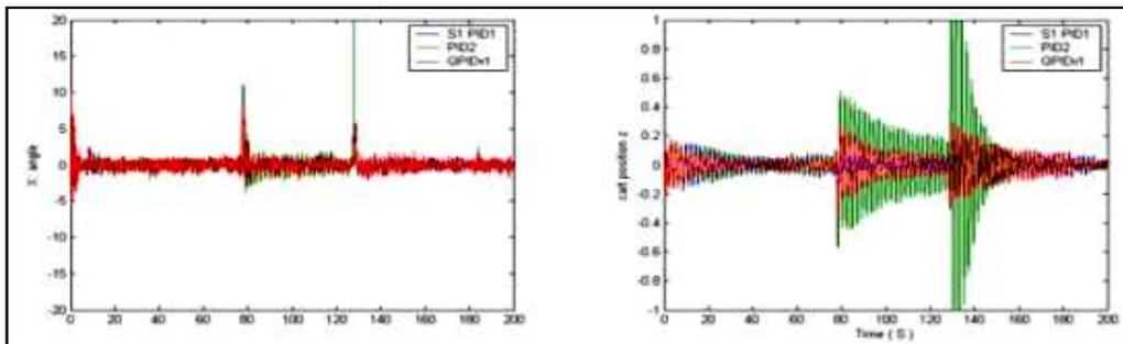
**Figure 16. Pole motion (left) and cart motion (right) comparison in New 1 situation**
