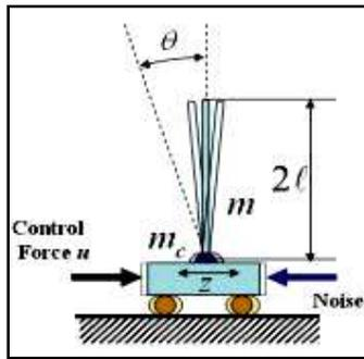
Figure2. Geometrical model of cart-pole system
